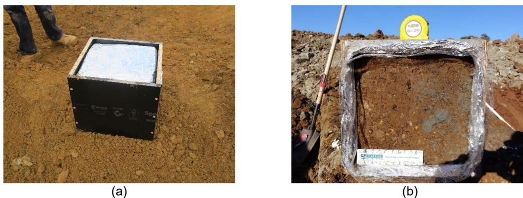
Figure 3: Partially wrapped block prior to spraying foam (a) and the base of a block prior to final wrapping (b)
