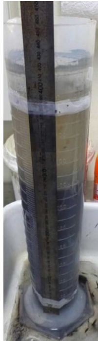
Figure 3: Simple column settling test
