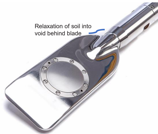
Figure 12: View of DMT highlighting void space in close proximity to sensor
