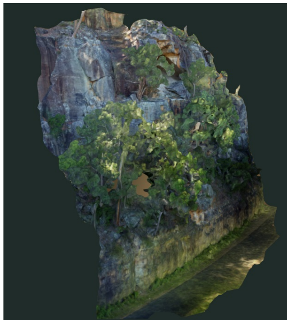
Figure 5. 3D model of cliffs captured by UAV photogrammetry
