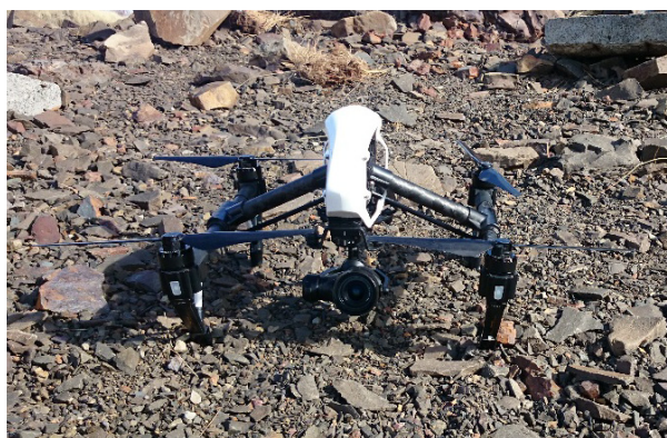
Figure 1. Quad-rotor mini UAV system carrying a high resolution camera.
