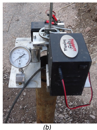
Figure 1. (a) Typical Borehole Shear Test Apparatus (Handy, 2013); and (b) Photo of the BST with retrofitted motorised crank during a trial test in a cased borehole.
