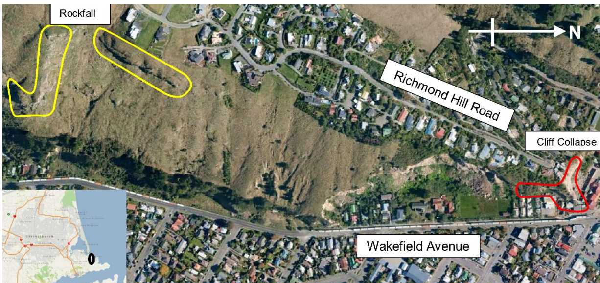
Figure 1. The rockfall and cliff collapse hazards affecting Wakefield Avenue are indicated in yellow and red respectively. (Image courtesy of Google Earth Pro, 30 June 2016).
