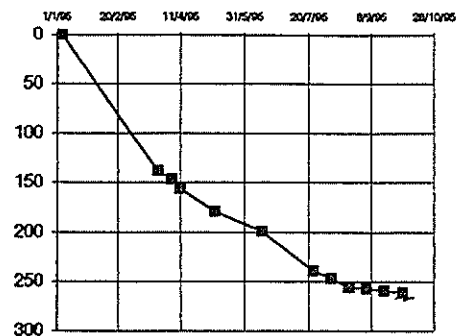
Plate 10: Total Predicted Settlement Approximately 300mm
