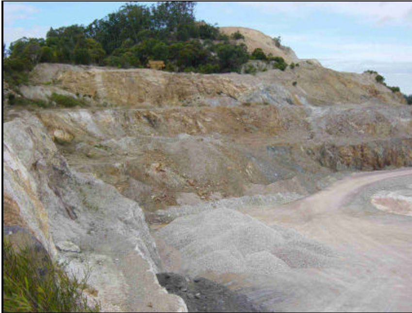
Figure 2: Picture of N-E Face with exposed carbonaceous shale (Acid Hot Spot)
