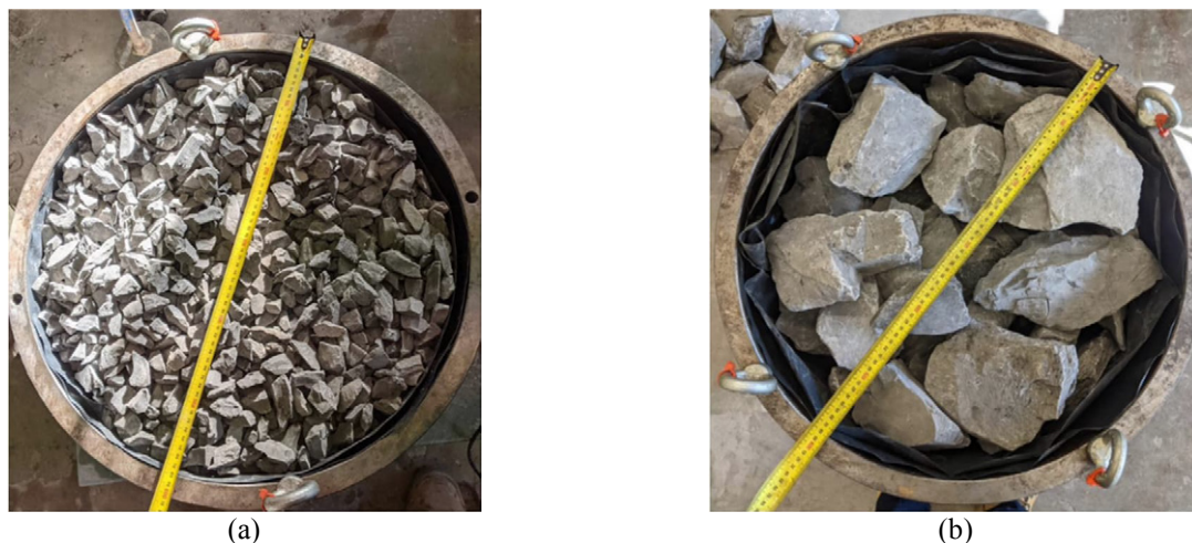
Figure 7 Dry sample of massive siltstone used for scaling effect compression tests. a) 19-26 mm, b) 150-200 mm
