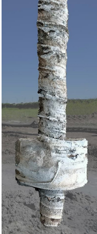
Figure 10: PAILE formed in fill
