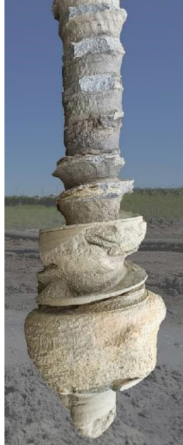
Figure 11: PAILE formed in loose to medium dense sand
