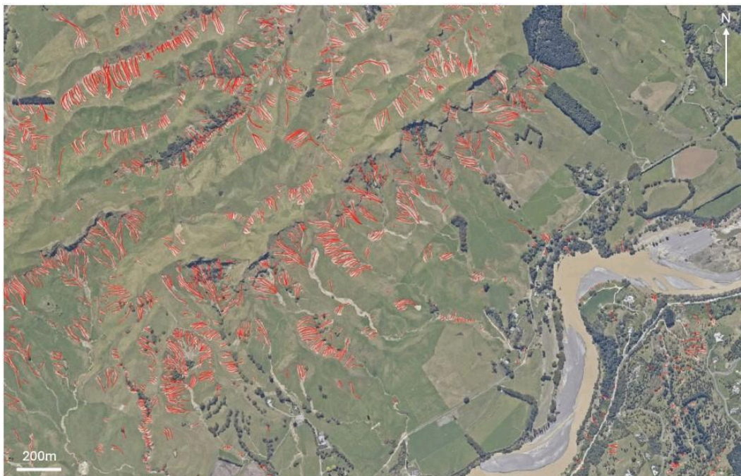
Figure 1: Extract of Landslide Runouts (red) in Study Area. Tukituki River, Hawkes Bay. Aerial Photograph downloaded from LINZ and captured between 19-21 February 2023.
