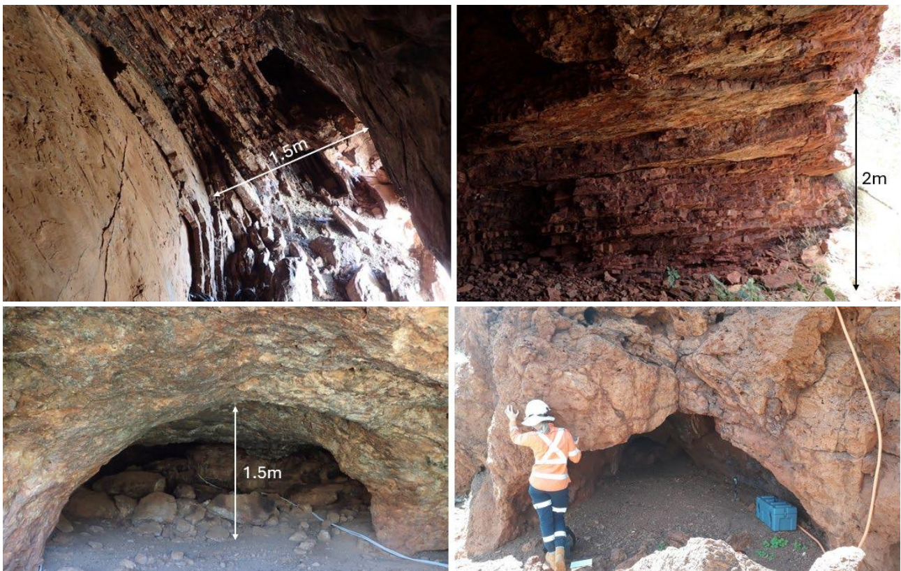
Figure 2 - Top: Examples of caves formed on steeply (left) and shallowly (right) dipping bedding. Bottom: Examples of caves formed in hydrated BIF rock mass.
