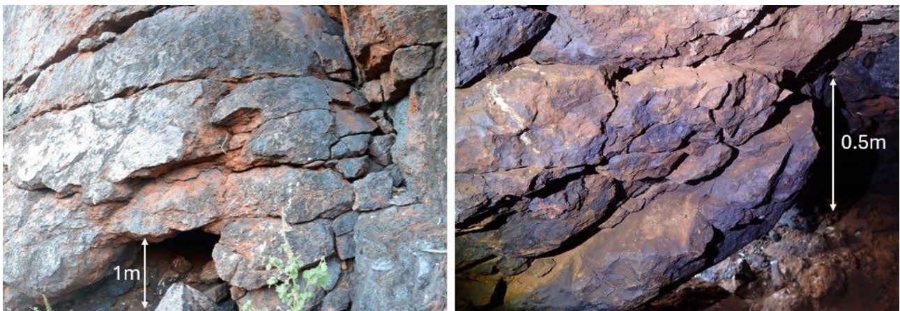
Figure 11 - A cave entrance viewed from outside and inside, showing dilated, blocky, loosened rock mass. Daylight was visible through the defects from the inside.
