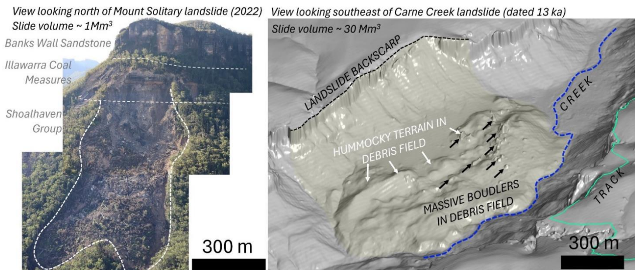
Figure 7: Examples of very large recent and ancient rock and debris slides with volumes exceeding 1 Mm 3
