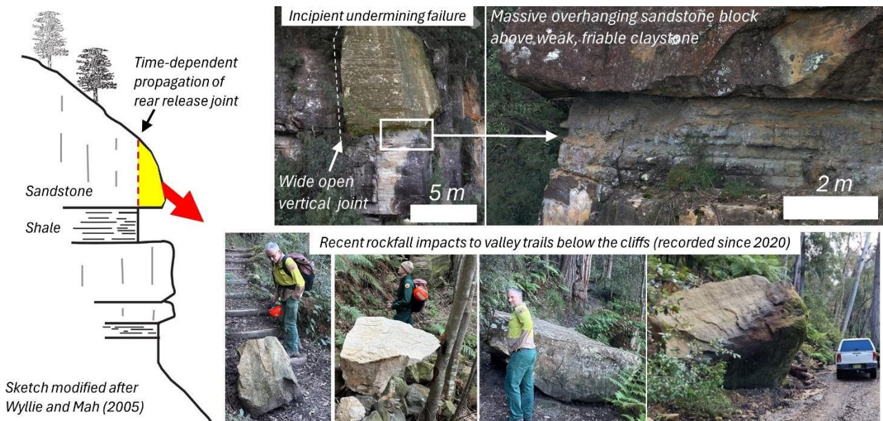
Figure 4: Conceptual sketch of time dependent rockfall initiation and examples of recorded rockfall impacts
