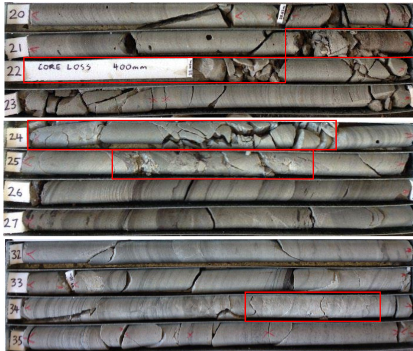
Figure 2: Examples of structurally deformed, fresh Hawkesbury Sandstone from within the published LPFZ as highlighted. Borehole SRT_BH070 completed as part of the projects tender phase site investigation program.
