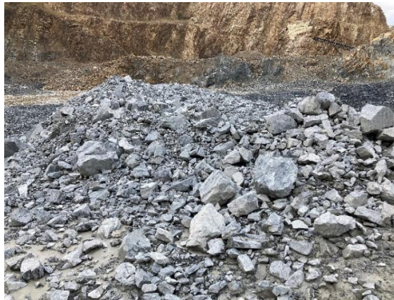
Photograph 1 - Blast pile of SW to FR argillite from Woolgoolga quarry within Coramba formation (Ccoc)
