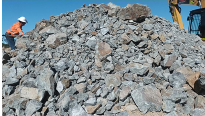
Photograph 5 - Material to be used for unprocessed rockfill trial
