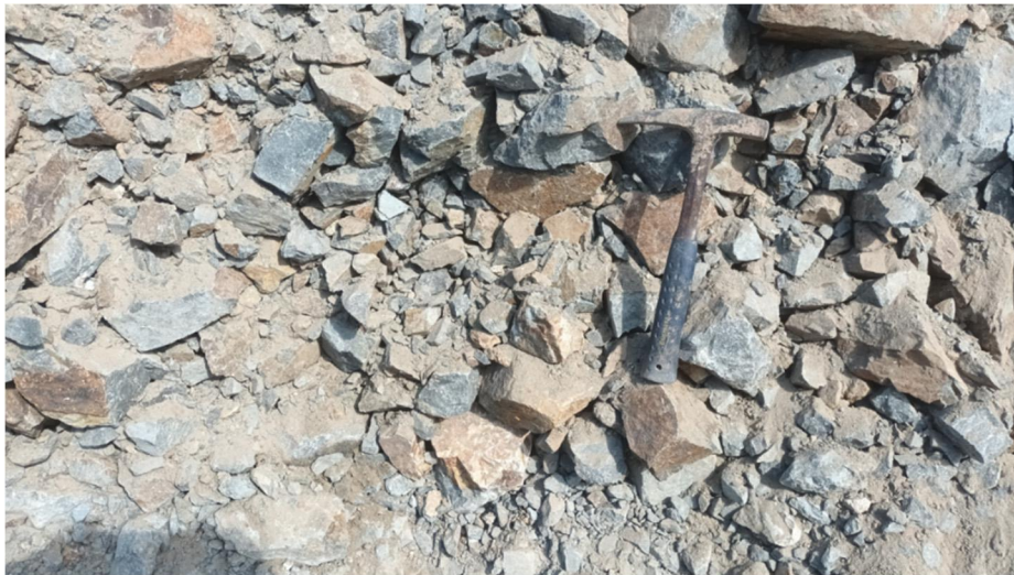
Photograph 7 – Particle size distribution and mechanical interlock exposed in Trial 1 test pit.
