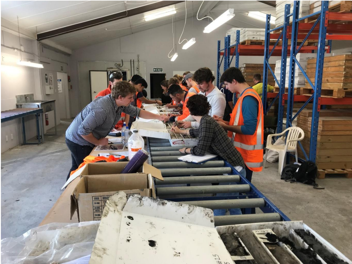
Figure 4: Logging Te Kuiti Group rock core in the core shed at Rotowaro mine using the NZGS (2005) guidelines
