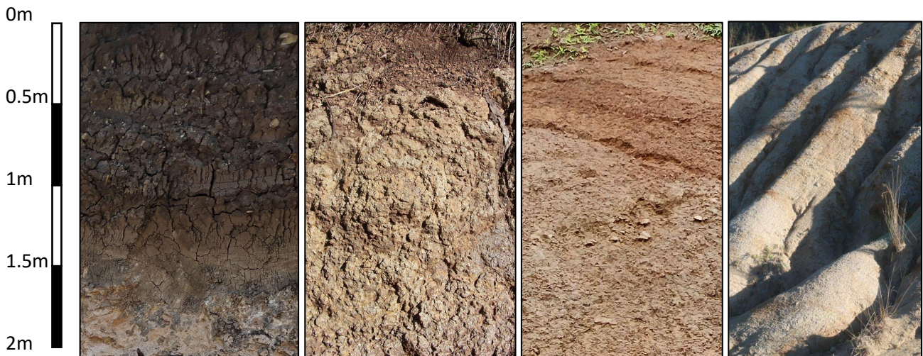
Figure 1. Four weathered basalt profiles: highly plastic clay (left); crumbling friable rock (middle); tuff (right).
