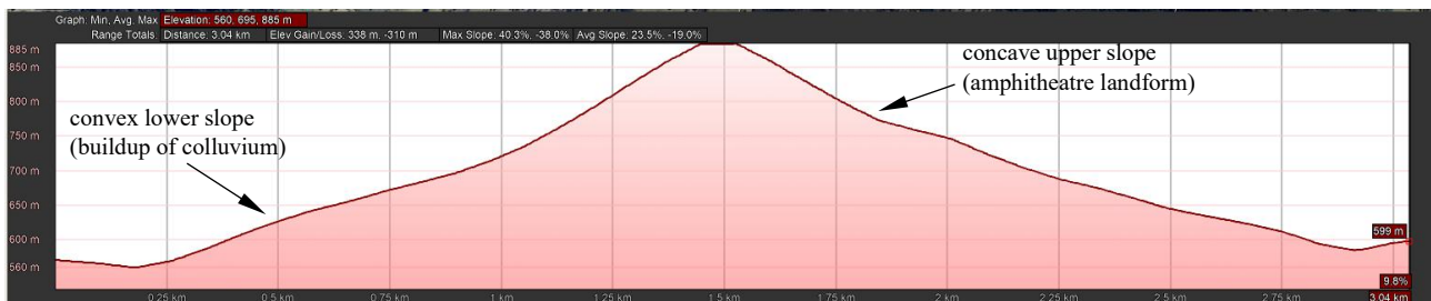
Figure 2. Ground profile through a basalt ridge extending from the Great Dividing Range, Murrurrundi.
