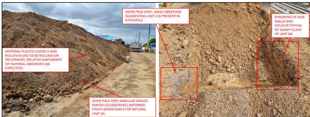
Figure 4: Site photographs of stockpiles and excavated test pits within the stockpile (with commentary).
