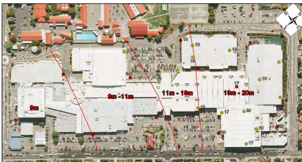
Figure 2: Northlands site plan showing approx. depth to dense gravel
