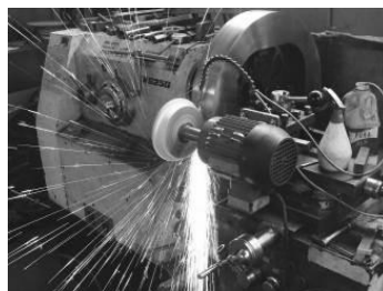
Figure 7b: Grinding outside of reaction ring
