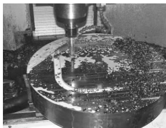
Figure 7a: The removal of the centre of the original blank slab
