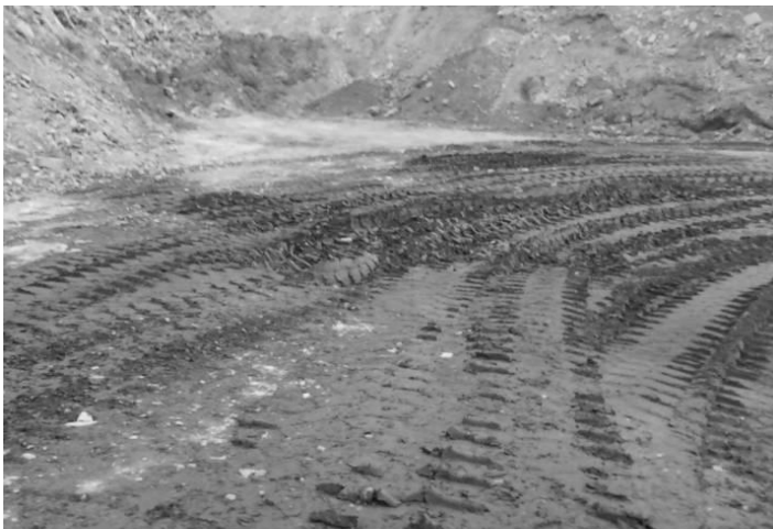
Figure 4, Dump truck tracks bogging in stope fill
