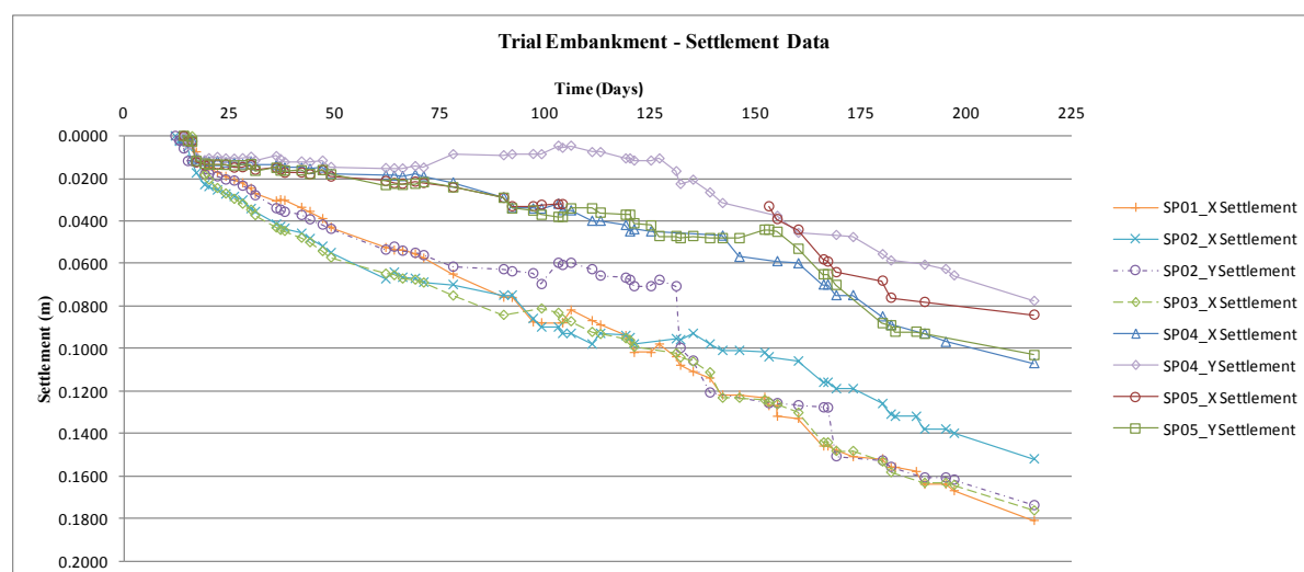
Figure 3: Magnitude of Settlement – Trial Embankment Settlement Plates
