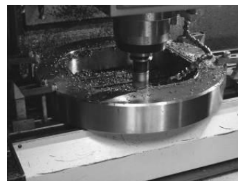
Figure 7c: Finishing the inner surface of the reaction ring
