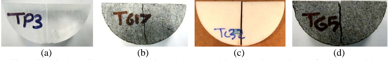
Figure 3: A single tensile crack observed in loaded truncated Brazilian disc specimens of brittle materials including polymethyl methacrylate (PMMA), granite, ceramic and basalt
