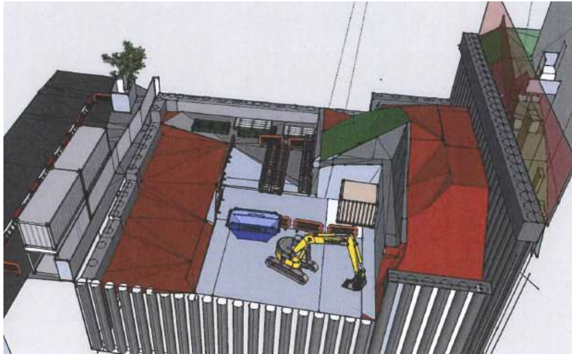
Figure 9: Construction of perimeter pile wall and capping beam
