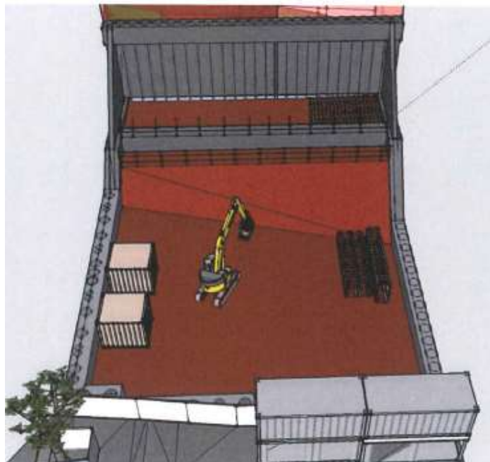
Figure 10: Excavation to Diaphragm Slab level
