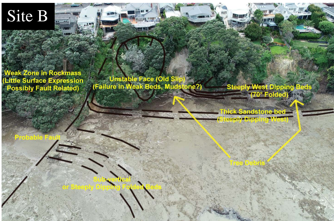
Figure 2: Examples of terrain evaluations produced from UAV photography. Site A) Typical soil failure observed along cliff tops in the Auckland Area. Site B) The variability of the East Coast Bays Formation geologic structure, the influence of the underlying geological structure of soil failures is important (Moon and Healy, 1994).
