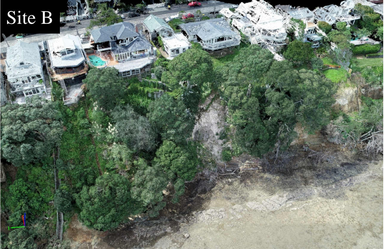
Figure 3: 3D models produced from the UAV aerial photography, from these models it is possible to gain a new perspective of the site and the underlying geological issues, in addition to allowing the creation of accurate cross-sections for stability analysis.
