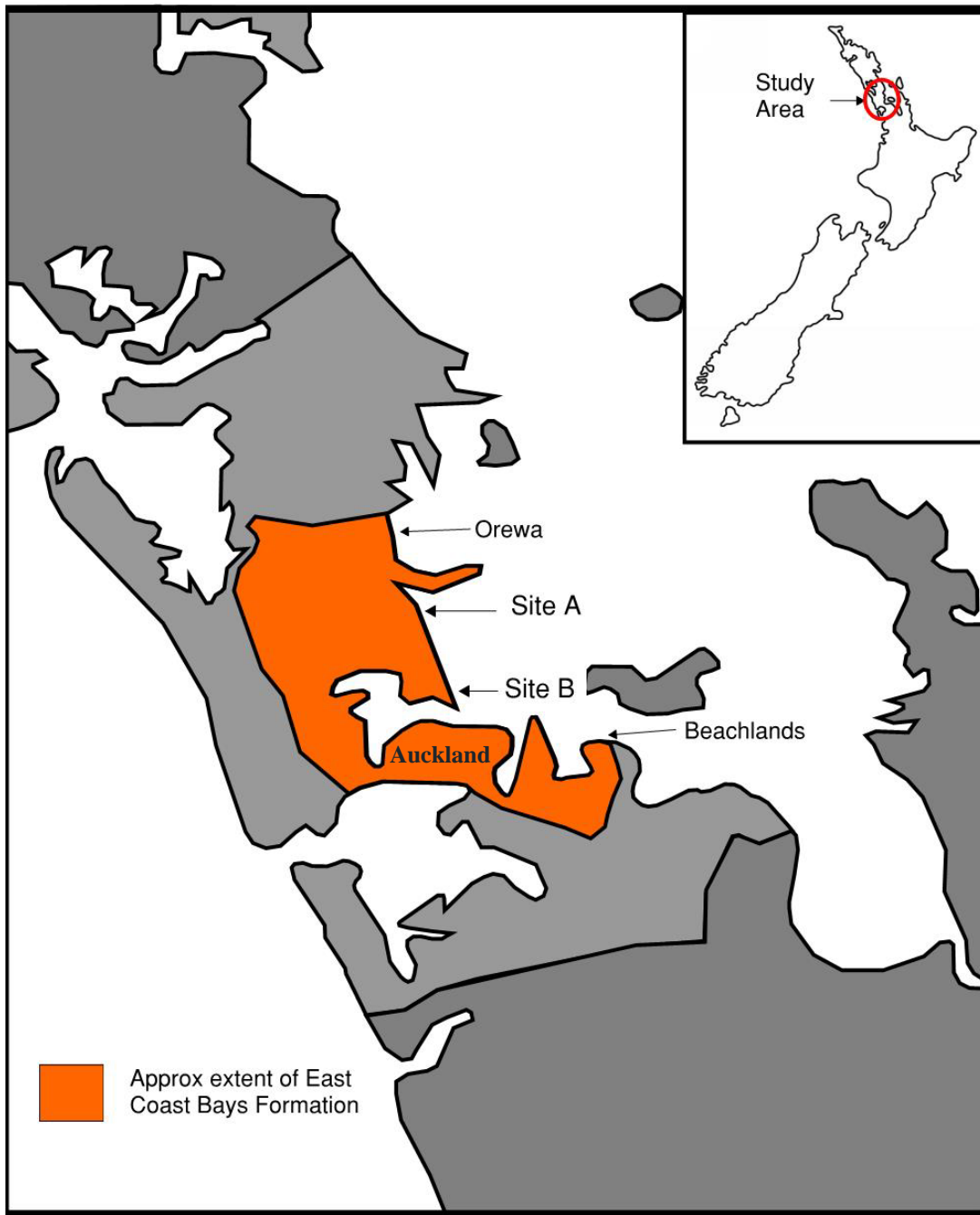
Figure 1: Simplified geological map of the Auckland Region, showing the approximate extent of the East Coast Bays Formation outcrops. The formation underlies the majority of the Auckland urban area.
