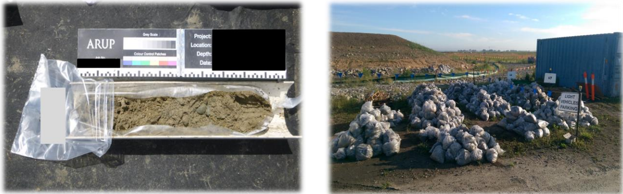
Figure 3: Photographs of PCV utilised to control soil and fluids whilst overwater (left) and stockpiled sonic core samples with each pile representative of a single day return (right)
