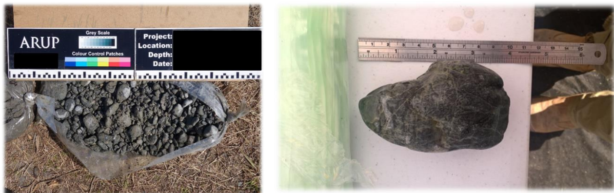
Figure 2: Example sonic soil core containing gravel and cobble material (left) and recovered cobble stone (right)
