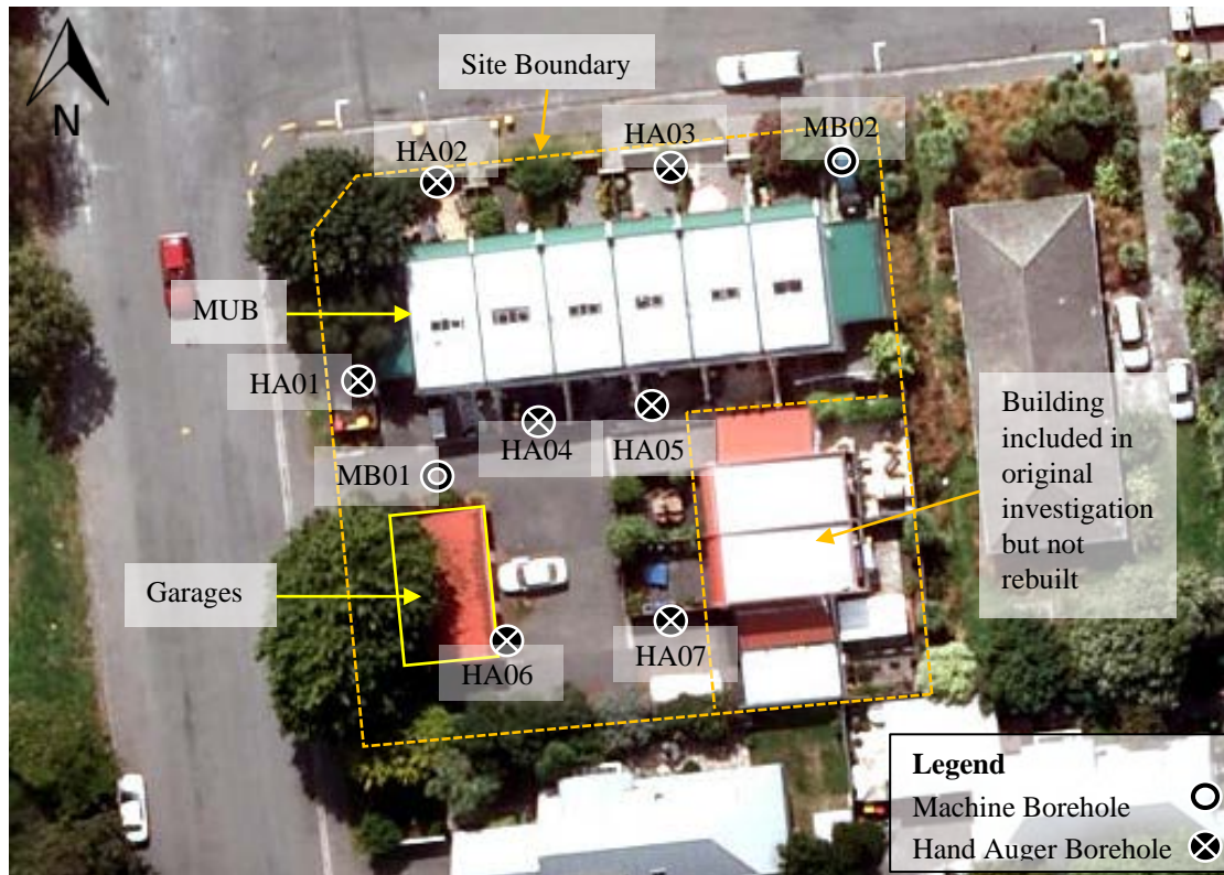
Figure 1: Site layout at the time of the 2014 investigation including the hand auger boreholes and machine borehole locations (aerial imagery sourced from Canterbury Maps, not to scale).
