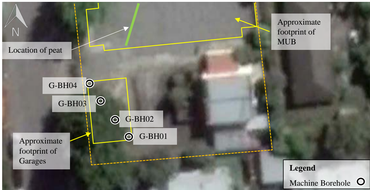
Figure 5: Location of additional machine boreholes within the garage footprint (October 2017 aerial imagery sourced from Google Earth, not to scale).
