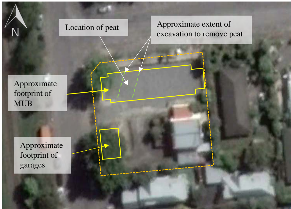
Figure 3: Location of encountered peat material (October 2017 aerial imagery sourced from Google Earth, not to scale).
