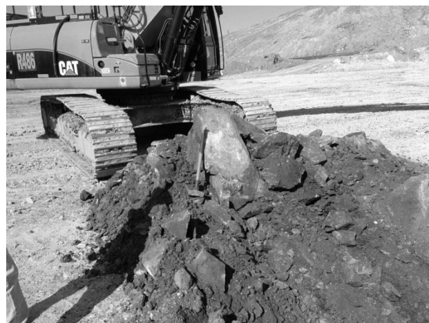
Figure 2. Typical excavated mine spoil, including oversize material. A ten-pound sledge hammer can be seen at centre as a scale reference
