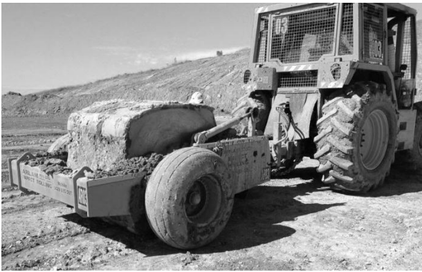
Figure 3. Four-sided impact roller pulled by mine specification agricultural tractor
