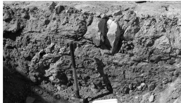
Figure 4. Side wall of test pit showing typical mine spoil material. A ten pound sledge hammer has been placed in the foreground for scale
