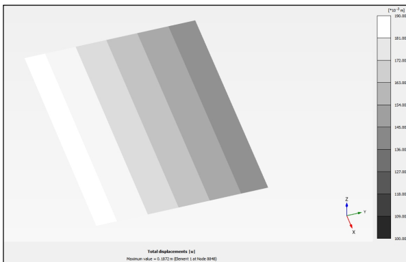
Figure 4(c). Differential settlement in right side footing.
