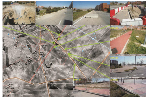
Figure 3. Damage Inventory, over 1956 aerial photo, showing ancient gypsum excavations, collapses, and linear incisions in the study area.
