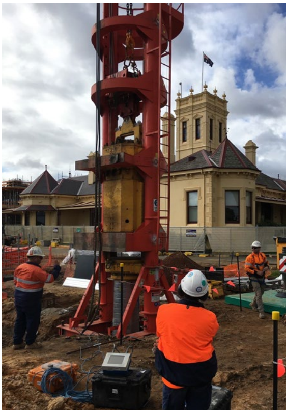
Figure 10. Example of a large drop hammer used to dynamically test a built-up CFA pile.
