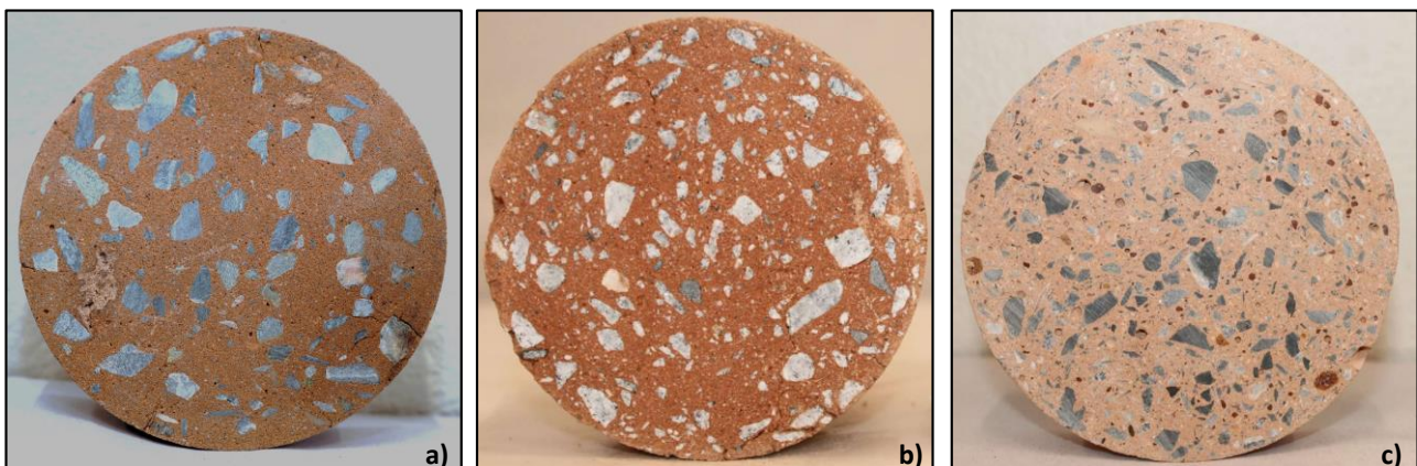
Figure 8: Cross section of view of UCS specimen following testing for a) Cosmos, b) Forrestania and c) Nova Mines
