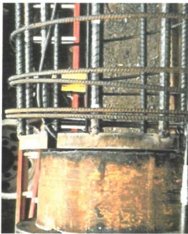
Figure 11. Fibre optic sensor placed along reinforcing bar.
