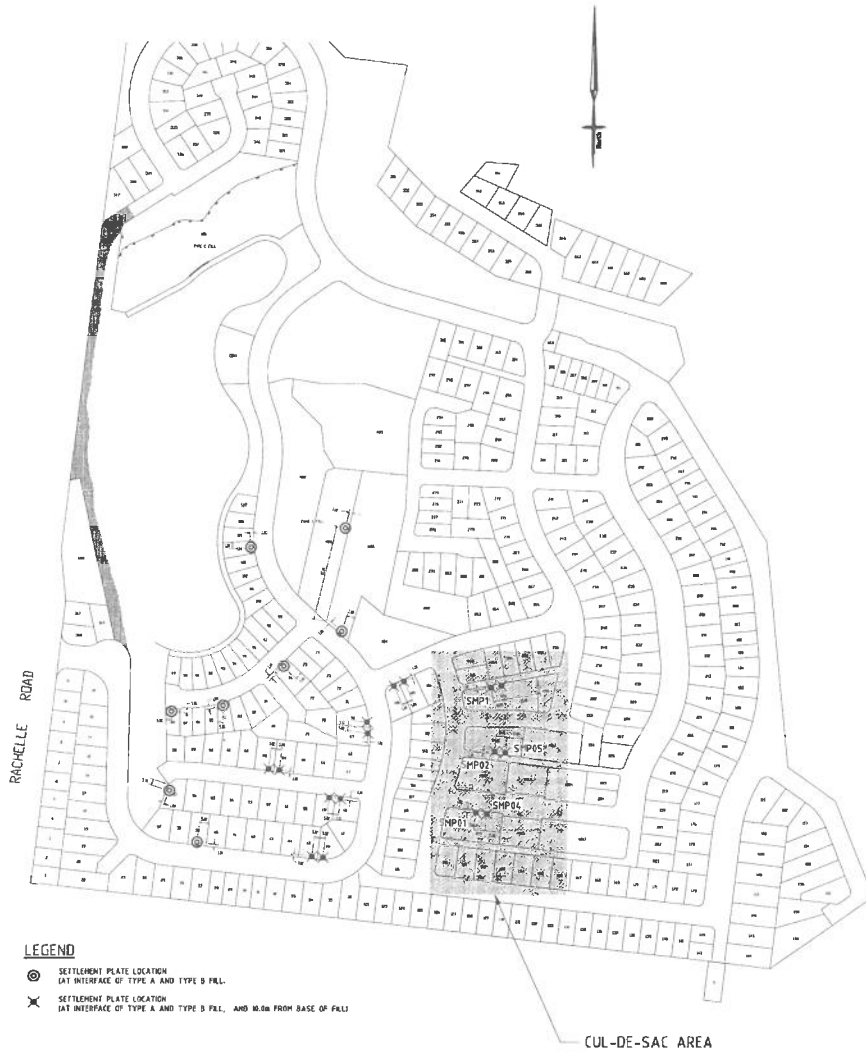
Figure 6 Cul-de-sac Settlement Monitoring Plate Locations
