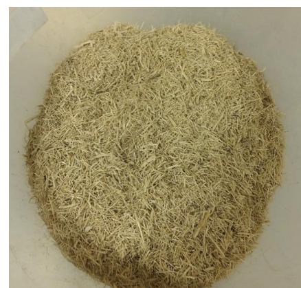
(b) Bagasse fibre (length: 0.3 mm to 13.8)
