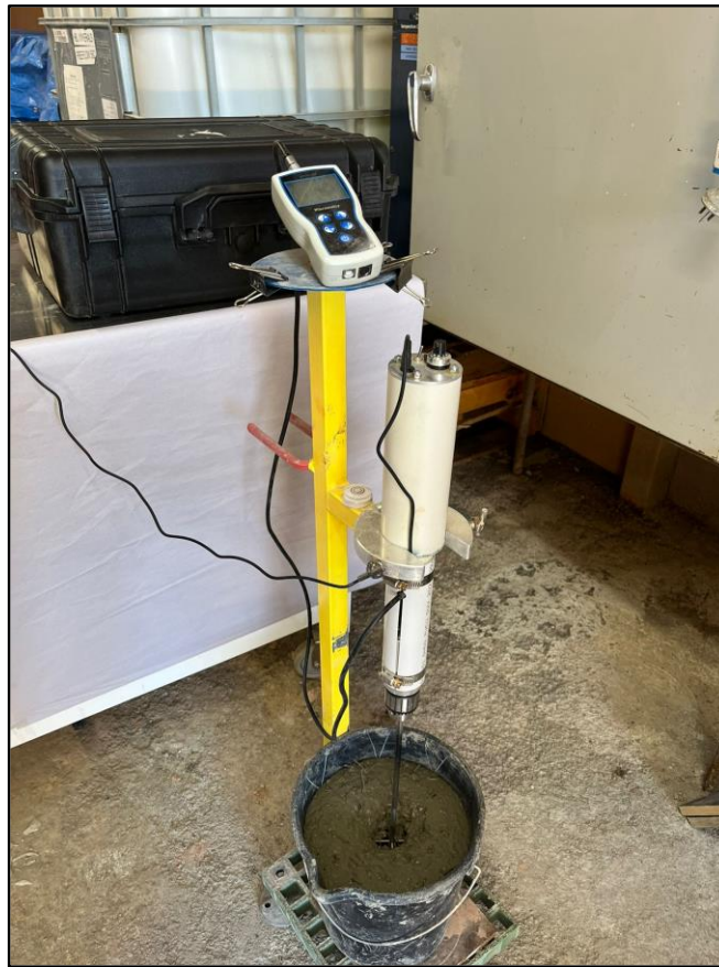
Figure 4: A large-scale viscometer used to determine yield stress of full shotcrete mixes
