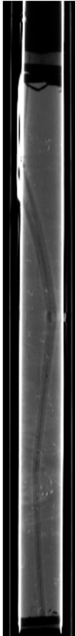
Fixed Piston sampler ( \phi=63 mm)
