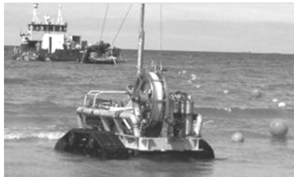
Figure 5b. Lankelma (UK) Subsea Crawler (working in surf zone)
