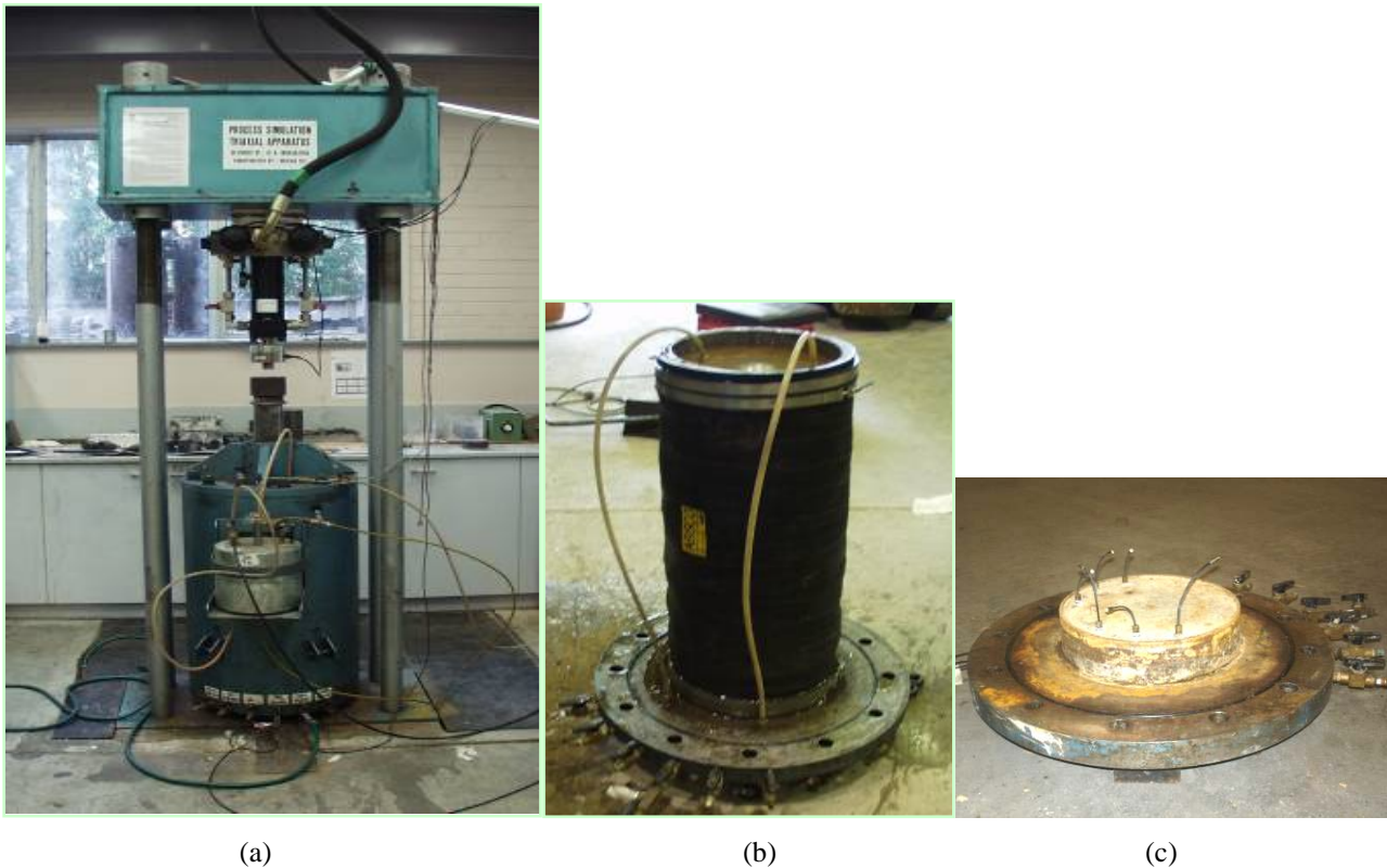
Figure 1: (a) Large-scale triaxial apparatus, (b) Soil specimen and (c) Miniature pore pressure transducers.
