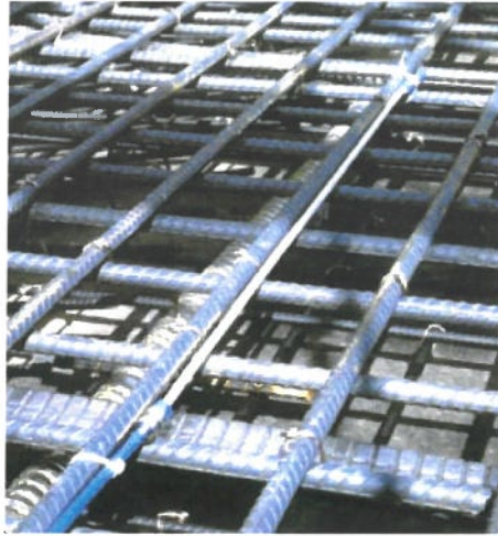
Figure 11. Fibre optic sensor placed along reinforcing bar.
