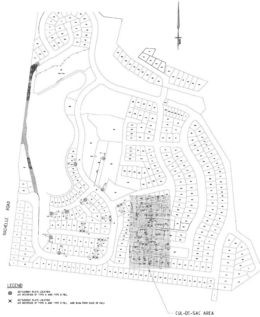
Figure 6 Cul-de-sac Settlement Monitoring Plate Locations
