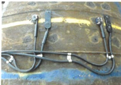
Figure 14. Dynamic pile testing instrumentation.
