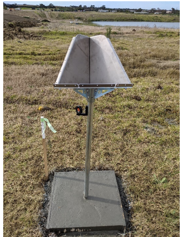
Figure 3. InSAR reflector installed at the SRL stabling yards (courtesy of Sixense Oceania).
