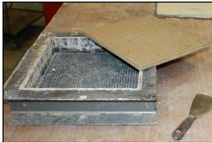
Figure 9: Casting mould and wooden plate covered by steel mesh.
