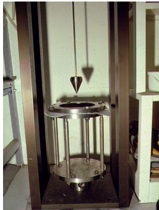
Drop weight test – 1kg sharpened cone
