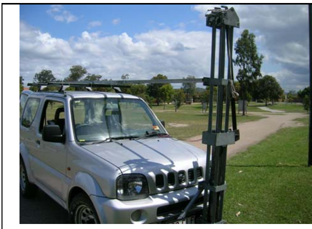
Figure 4: A vehicle-mounted weight dropping system.
