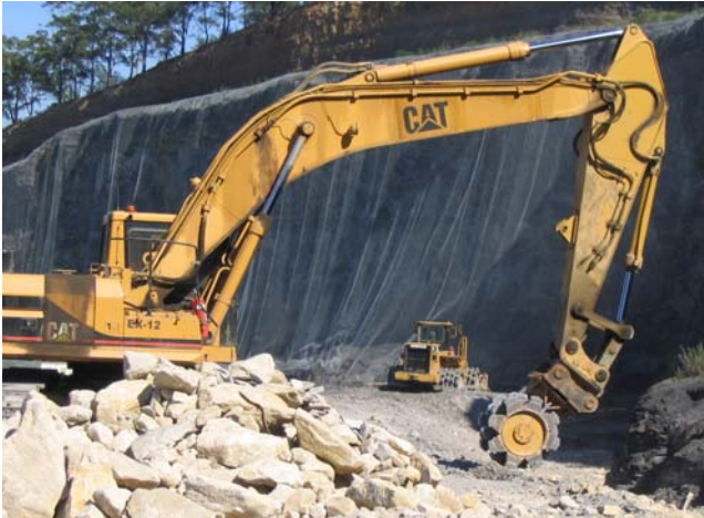
Figure 9: Pad foot wheel trench backfill compactor.
