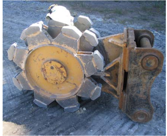
Figure 10: Pad foot wheel roller.
