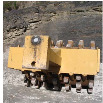
Figure 12: Modified towed pad foot roller.
