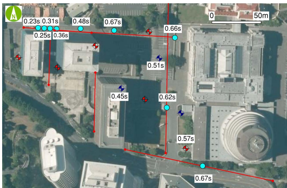
Figure 9: Locations of the ReMi seismic arrays and boreholes (red) at Bowen Campus/Parliament Precinct, Wellington, New Zealand. Site period measurement values across the site are presented, with estimates from the seismic ReMi data shown as cyan circles. Aerial photograph sourced from LINZ Data Service ( https://data.linz.govt.nz/data/category/aerial ) and licenced under the Creative Commons Attribution 4.0 New Zealand.
