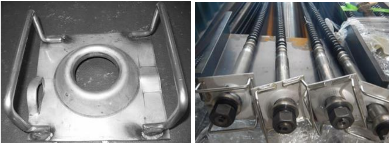
Figure 5: Handle-bar face plate for rock bolts.
