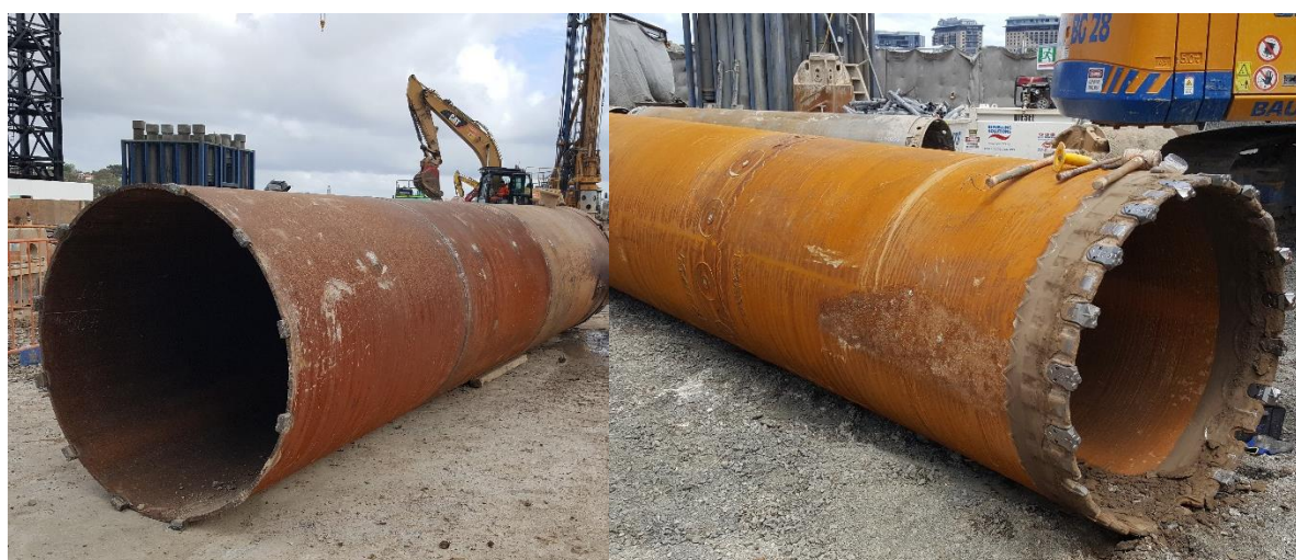
Figure 7: (left) Single wall casings with permanent teeth, and (right) double wall casing with interchangeable teeth
