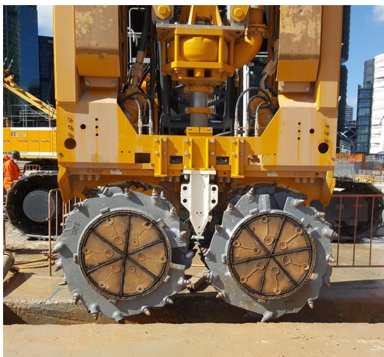
Figure 12: Hydraulic cutter with protruding teeth
