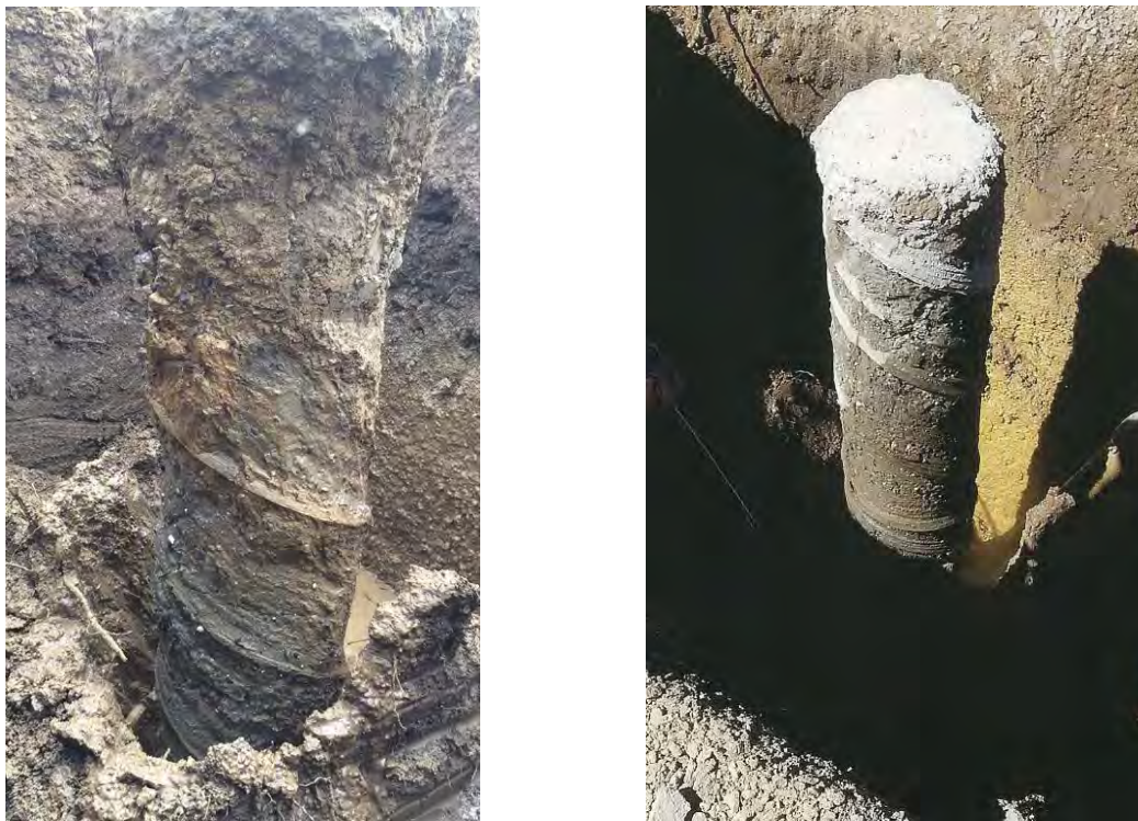
Figure 12 : Typical shape of excavated columns presenting sound characteristics
