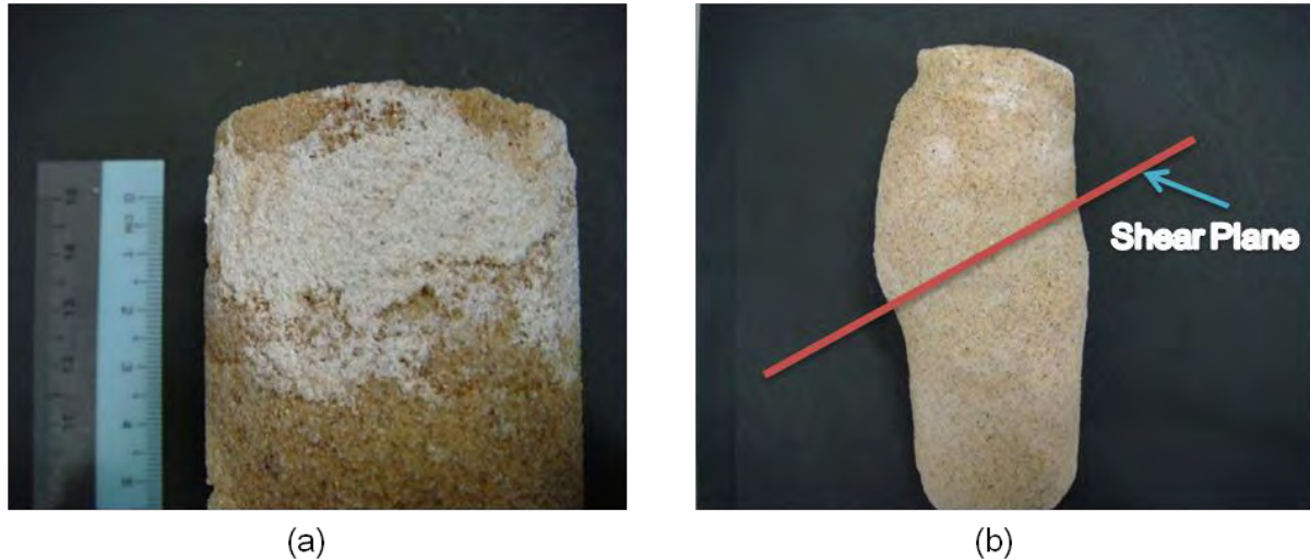
Figure 7: Samples retrieved from model test showing (a) sealing (b) welding effects.
