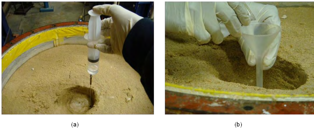
Figure 3: Foundation repair using (a) injection into surrounding sand and (b) pouring solution into the hole in the centre of the column.
