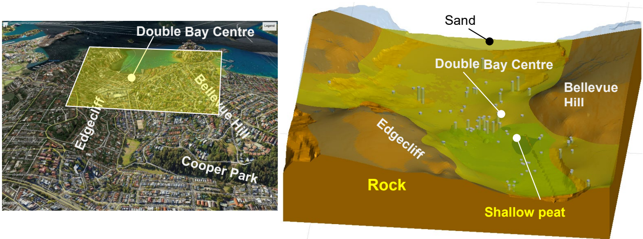
Figure 2: 3D geological model generated using Leapfrog software program
