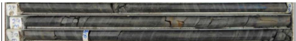
Figure 4: Photograph of section of core which contained a slickensided bedding plane which caused movement of a retention system shown in Figure 1
