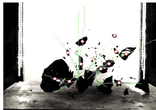
Figure 10. Post impact tracking of fragment trajectories (green lines) from high speed photographs (500 frames per second).
