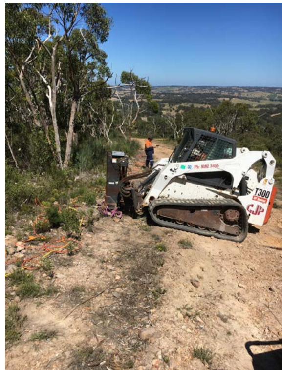
Figure 2. Bobcat T300 with the drophammer and striker plate attachment in operation
