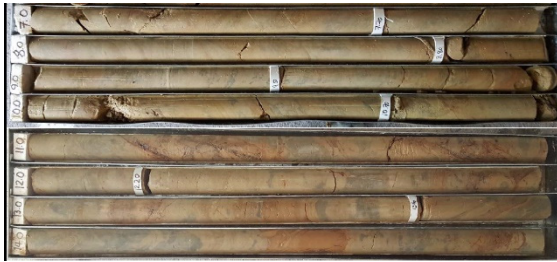
Figure 2. Example of typical highly to moderately weathered siltstone encountered at founding depth
