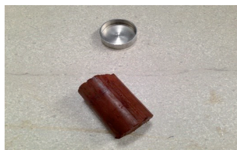
Figure 7: Sample B to be trimmed for suction testing
